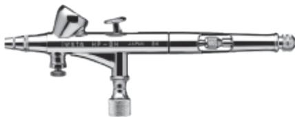
**Product Description:** The HP-BH offers ultimate air control directly at the nozzle with Iwata's Micro Air Control (MAC) Valve Technology. Designed for artists who demand extreme control of detailed spraying, this brush uses larger threads on the nozzle which offers a more secure hold and ensures better centering of the nozzle.
